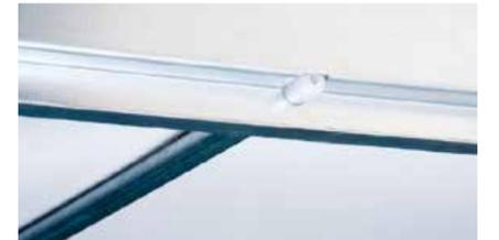
Cumberland's unique roller-guided manure belt system also supports low-wear operation in longer systems. Low rolling resistance reduces the required drive power, which increases the service life of the manure belt.
