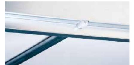
Cumberland's unique roller-guided manure belt system also supports low-wear operation in longer systems. Low rolling resistance reduces the required drive power, which increases the service life of the manure belt.
