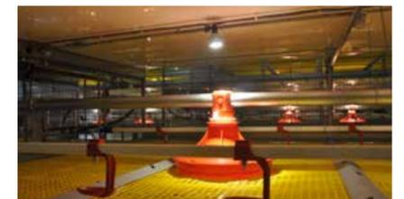
Optimal lighting for broilers with dimmable LED tubes or LED bulbs installed in the cage increases growth and feed conversion rate while keeping the birds comfortable.
